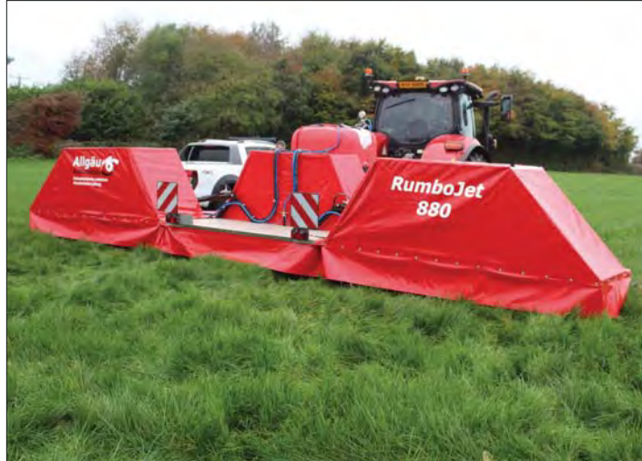
The RumboJet precisely spot sprays weeds within a grassland sward
